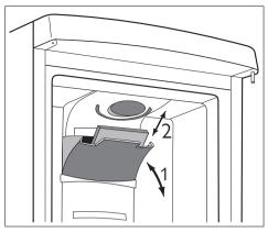
**Important!** During operation, always keep the air ventilation flap closed.
